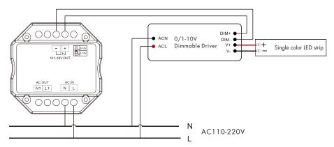
• Connect with 0/1-10V dimming driver (use AC OUT)
