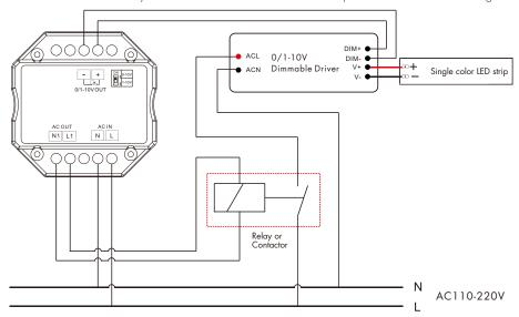
Note: We recommend the number of LED drivers connected to 0/1-10V dimmer does not exceed 100 pieces, The maximum length of the wires from dimmer to LED driver should be no more than 50 meters.
